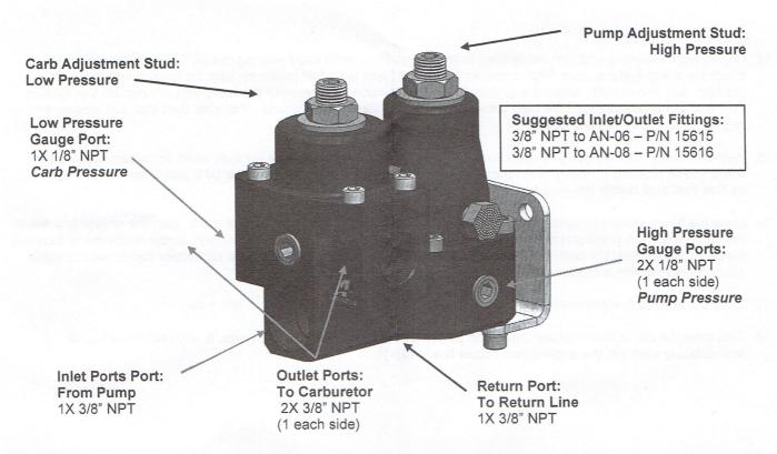
10. Attach the fuel return line to the regulator return port located on the **bottom** of the regulator, using a 3/8" NPT to AN-06 or barb fitting. Tighten all connections. **NOTE:** a return line **MUST** be used, routed from from the bottom (return) port, connected to the OEM return line, back to the top of the fuel tank.
